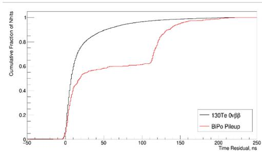
**Figure 1.** Cumulative timing classifier for Bi-Po pile-up events[2]. Signal events exhibit a smooth curve, but pile-up events show a step when the alpha decay occurs.
